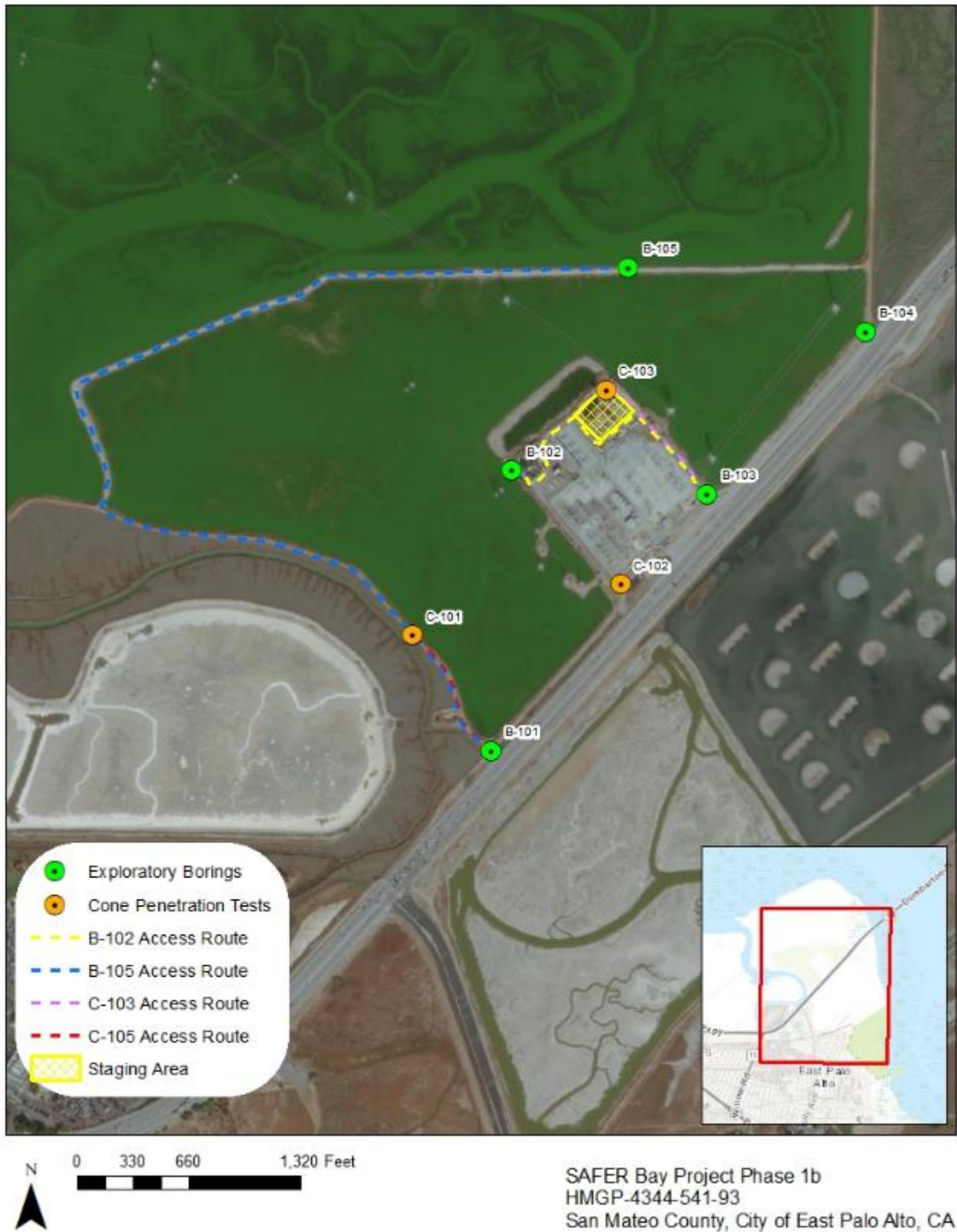
Figure 3a. Proposed Geotechnical Exploration – North project area
