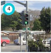
Kavanaugh Dr and University St: intersections with a history of disregarding signal violations can be reduced by upgrading signal equipment to larger signal heads reduce the frequency of collisions
