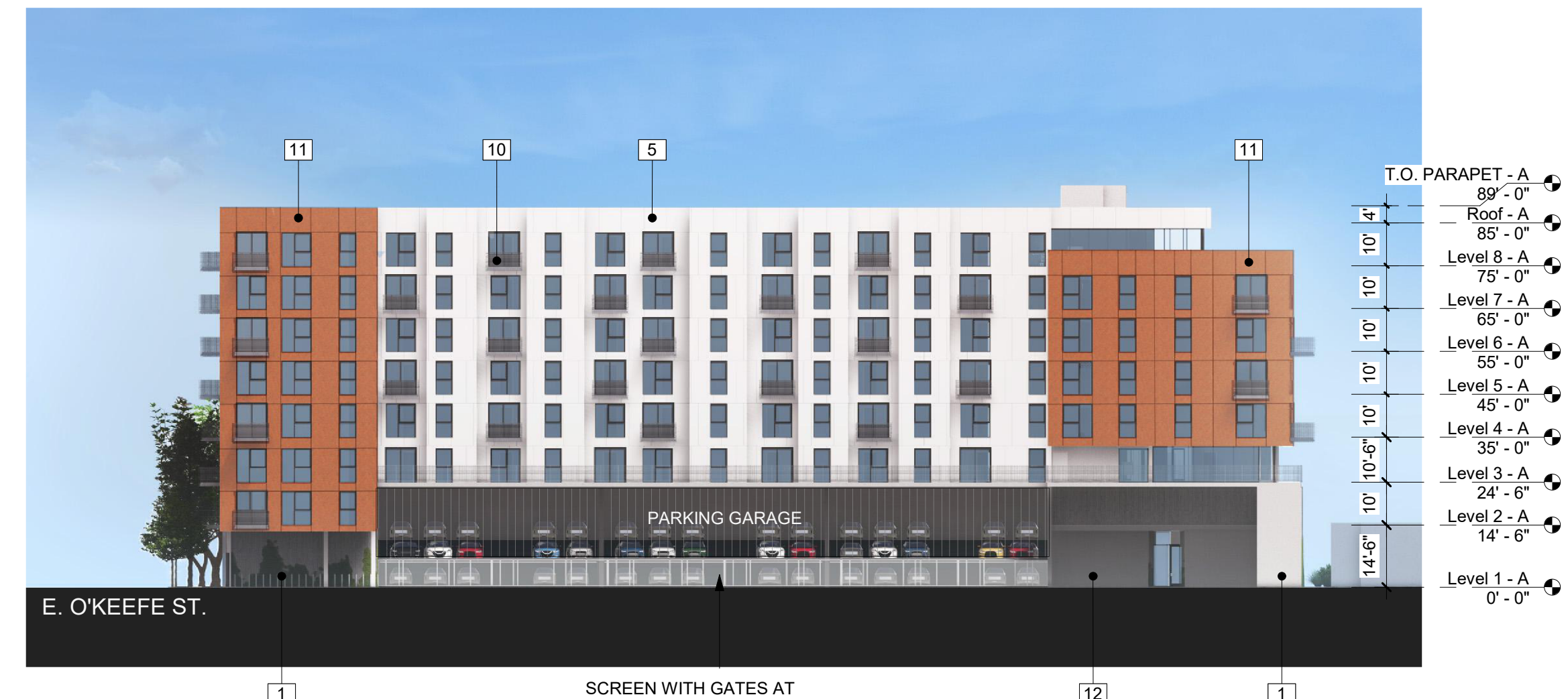
3 BUILDING A - WEST ELEVATION Copy 1 1" = 30'-0"
