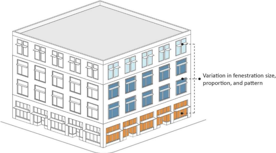
Figure 6-18: Examples of Base/Middle/Top Building Variation
